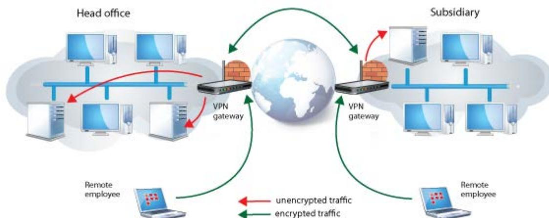
Figure 8: A VPN network scheme based on IPsec technology
